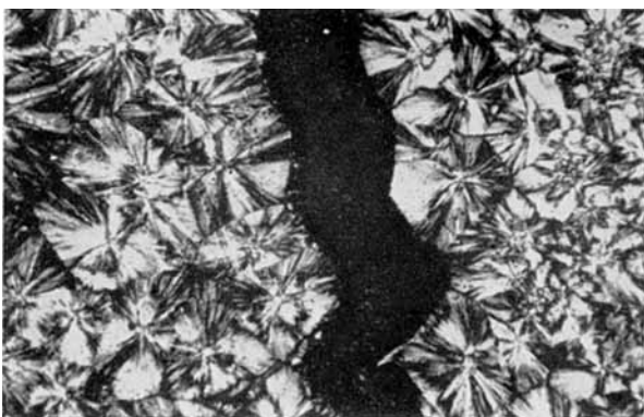
Fig. 6. Fracture of a completely spherulitic film (broken at high rate of speed).
